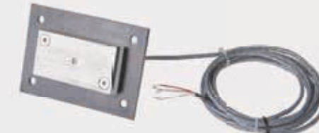
Rub-Block stainless steel belt misalignment sensor. 2 on each side in the elevator head section and 2 on each side in the elevator boot section
