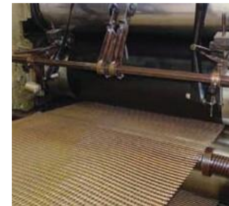
Polysur® Ferro SW-RE elevator belt during production
