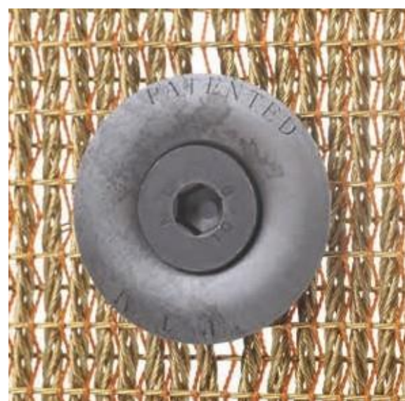
Bolt M12 with \varnothing 50 mm bolt head covers 25% more warp and weft cables than standard \varnothing 42 mm bolt head resulting in a stronger bucket to belt attachment.
