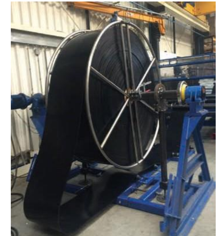
Decoiling the Polysur® Ferro belt in the CNC bolt hole drilling machine
