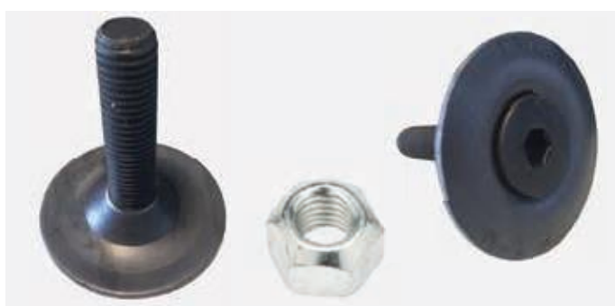
PTM style M12, 10.9 grade elevator bolt with \varnothing 50 mm bolt head and allen key. Complete with heat resistant M12 DIN 980V locknut.
