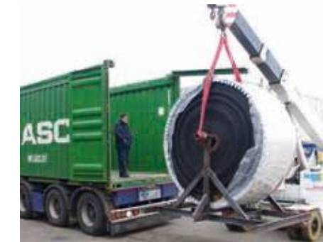
Loading a 8.2 tons Polysur® Ferro elevator belt with crane in a 20' open top high cube container
