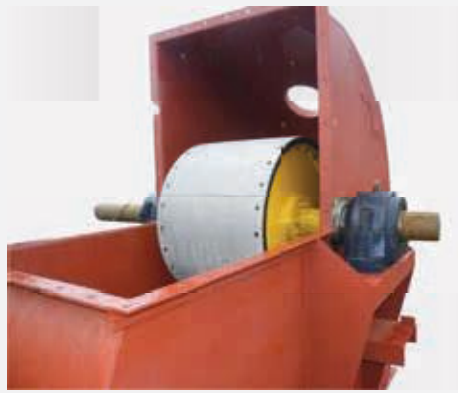
Elevator head section with drive pulley with 'Metallag' sintered all metal pulley lagging
